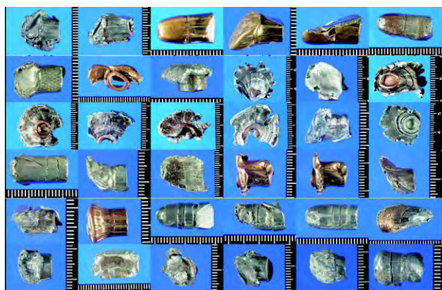
Fig. 11 Evidence Bullets Many evidence bullets were deformed badly as they were fired in high speeds.
