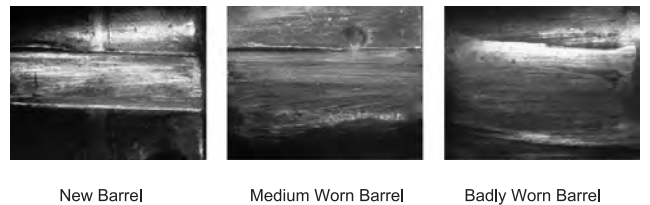
Fig. 5 Landmarks Fired from Tokarev Semi-automatics
