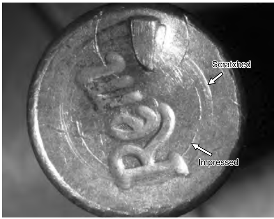
Fig. 2 Scratched Mark and Impressed Mark
