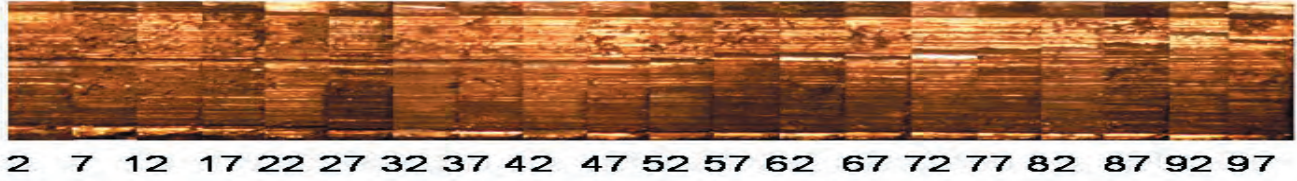
Fig. 13 Reproducibility of prominent striations on landmark 1 of Frangible 115 grain bullets. Note that the relative position of these striae to the driving edge was shifted toward the direction of the trailing edge in accordance with successive firing. This photo was made by overlaying segments of photos which were cut from bullet base areas.
